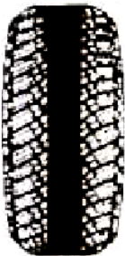
Too high air pressure
